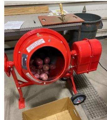
**Figure 2. Cement mixer setup for evaluating tuber skinning.**
