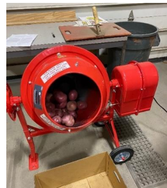
Figure 2. Cement mixer setup for evaluating tuber skinning.
