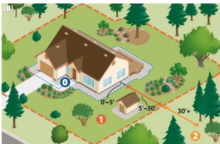
*This diagram shows proper density and spacing of plantings in the ember ignition zone (0); lean, clean and green zone (1); and reduced fuel zone (2).*
