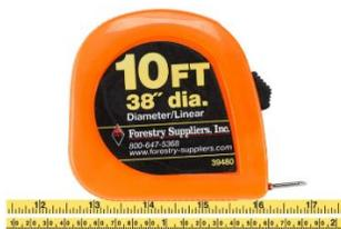
Used to measure the diameter of a tree at breast height (DBH = 4.5 feet up trunk from the ground) this tape has inches and feet on one side (which measures circumference), and on the other side measurements have been divided by pi to give you diameter.
