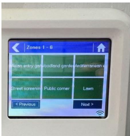
*Smart controller display showing six watering zones.*
