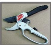
An anvil pruner has a top blade that closes down on top of a flat base, called the anvil jaw. The anvil is usually made of soft metal or hard plastic. The force makes cutting thick branches easier but tends to crush smaller plant stems.
