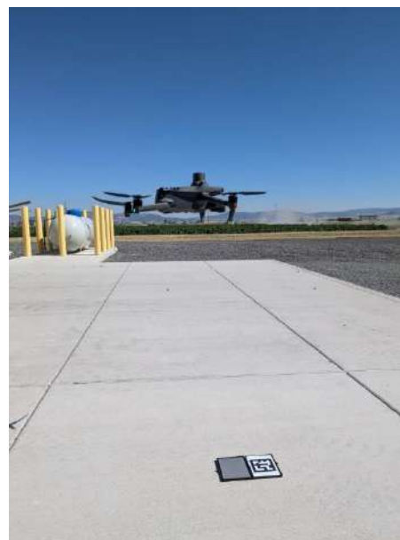
Figure 1: Capturing a drone image from the calibration panel.
